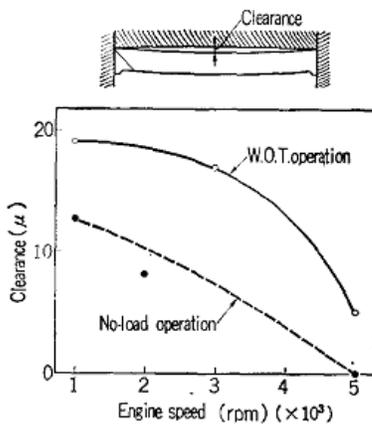
**Fig. 4.42** Clearance between apex seal and rotor housing
