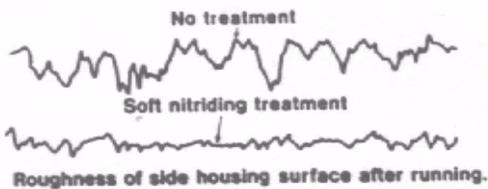
Roughness of side housing surface after running.
