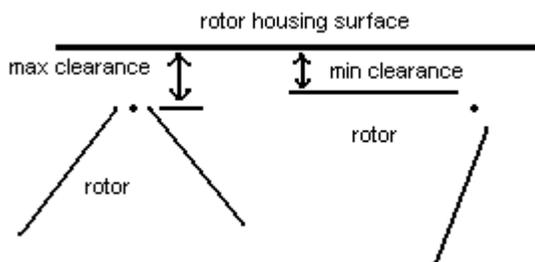
Although this sketch is not technically correct it helps to illustrate how the clearance changes as the angle of oscillation changes.
