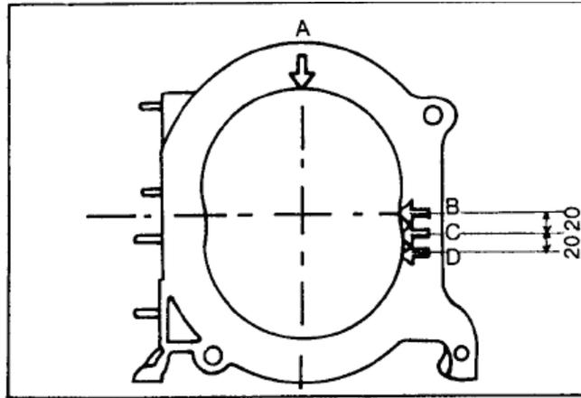
**Visual inspection after cleaning:** Once the part is clean, carefully inspect the rotor housing o-ring grooves to ensure that no grooves have been compromised due to excessive corrosion. Also inspect the water passages for corrosion.
